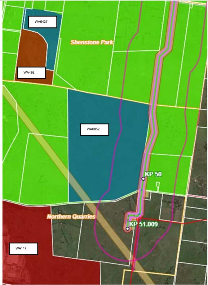
The pipeline passes the operational Barro Quarry WA492 and proposed extension area WA6437. At this point the pipeline is over 1.5km from the quarry and will not present any constraint to quarry operations.
